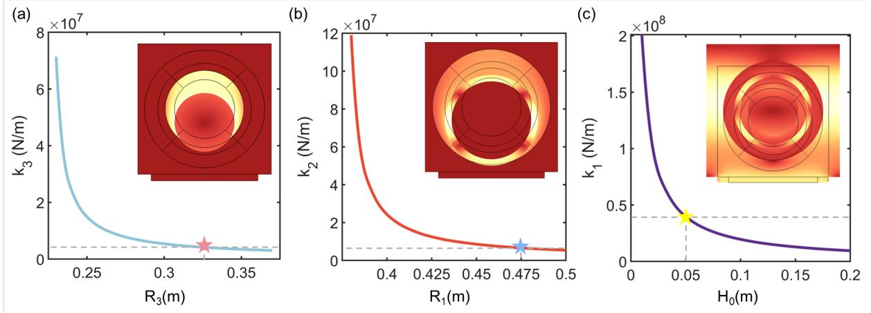
Figure 7: Stiffness of EDMs with three resonators ( $k_1$ ,  $k_2$ , and  $k_3$ ) under numerical tests and the optimal design corresponding to the actual structural geometry: (a) the intermediate resonator radius  $R_3$ , (b) the outermost resonator radius  $R_1$ , and (c) the element side length  $H_0$ .
