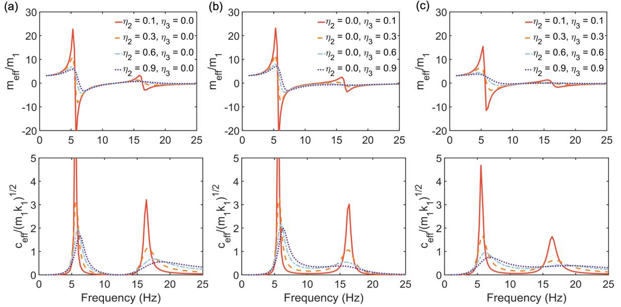
Figure 9: Effective mass and effective metadamping coefficient of EDM lattice system with three resonators with different loss factors: (a)  $\eta_2 = 0.1, 0.3, 0.6, 0.9$ ;  $\eta_3 = 0.0$ , (b)  $\eta_3 = 0.1, 0.3, 0.6, 0.9$ ;  $\eta_2 = 0.0$ , and (c)  $\eta_2 = \eta_3 = 0.1, 0.3, 0.6, 0.9$ .
