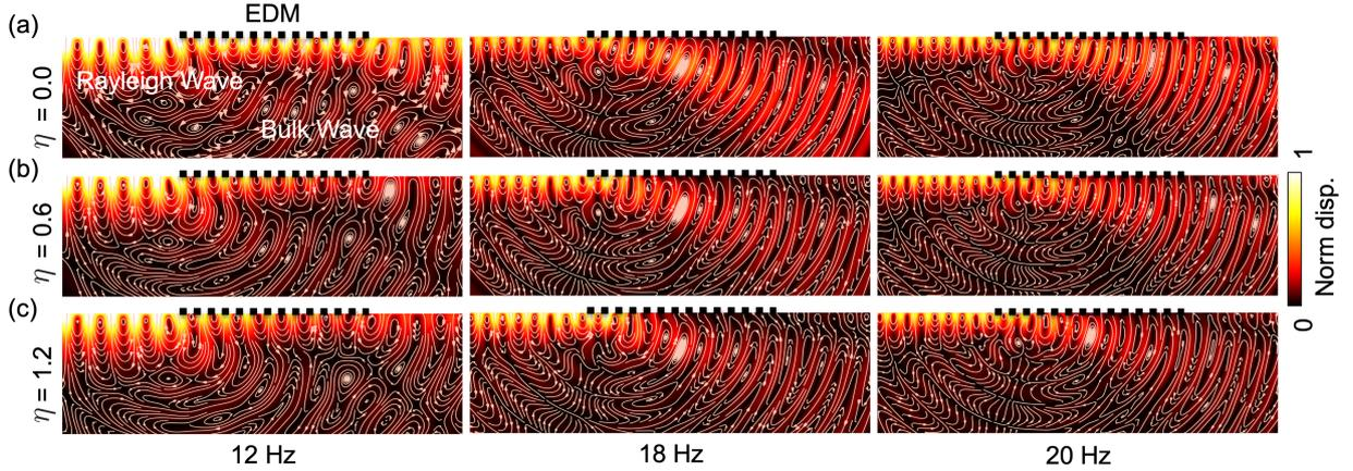
Figure 5: The wave scattering field of an incident Rayleigh wave at frequencies 12 Hz, 18 Hz, and 20 Hz, and loss factors (a)  $\eta = 0.0$ , (b)  $\eta = 0.6$ , and (c)  $\eta = 1.2$ .
