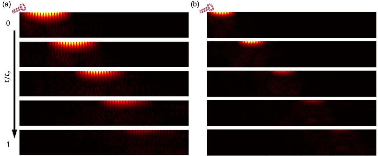
Figure 13: Verification of adiabatic evolution of Rayleigh waves in the **time domain**: (a) At 10 Hz. (b) At 18 Hz.
