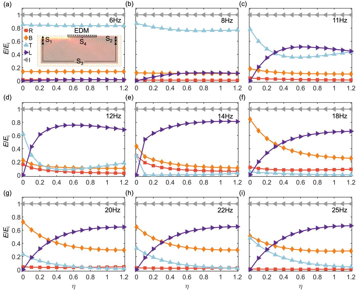
Figure 4: The energy ( $E$ ) normalized by the incident energy is categorized as reflected Rayleigh wave (R), transferred bulk wave (B), transmitted Rayleigh wave (T), resonator absorption (L), and incident wave (I) with respect to different loss factors and different frequencies.  $S_1$ ,  $S_2$ ,  $S_3$ , and  $S_4$  are the regions for calculating the energy of reflected Rayleigh wave, transmitted Rayleigh wave, bulk waves, and absorption by the EDM.
