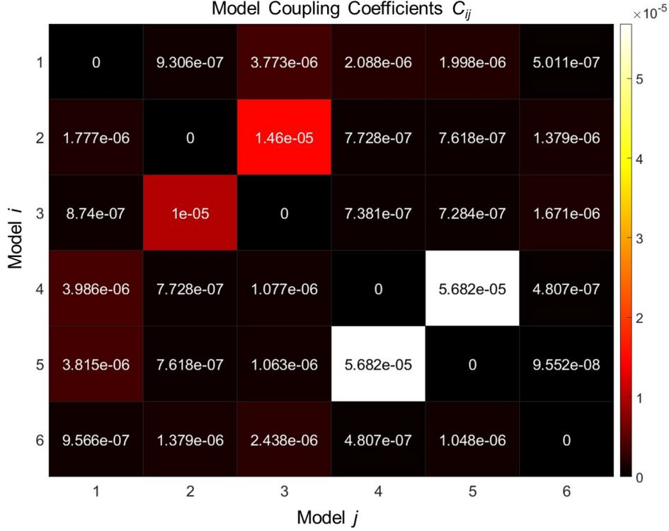
Figure 15: Mode coupling coefficients  $|C_{ij}|$  visualized as a heatmap. A system satisfying the adiabatic condition should exhibit near-zero off-diagonal elements.
