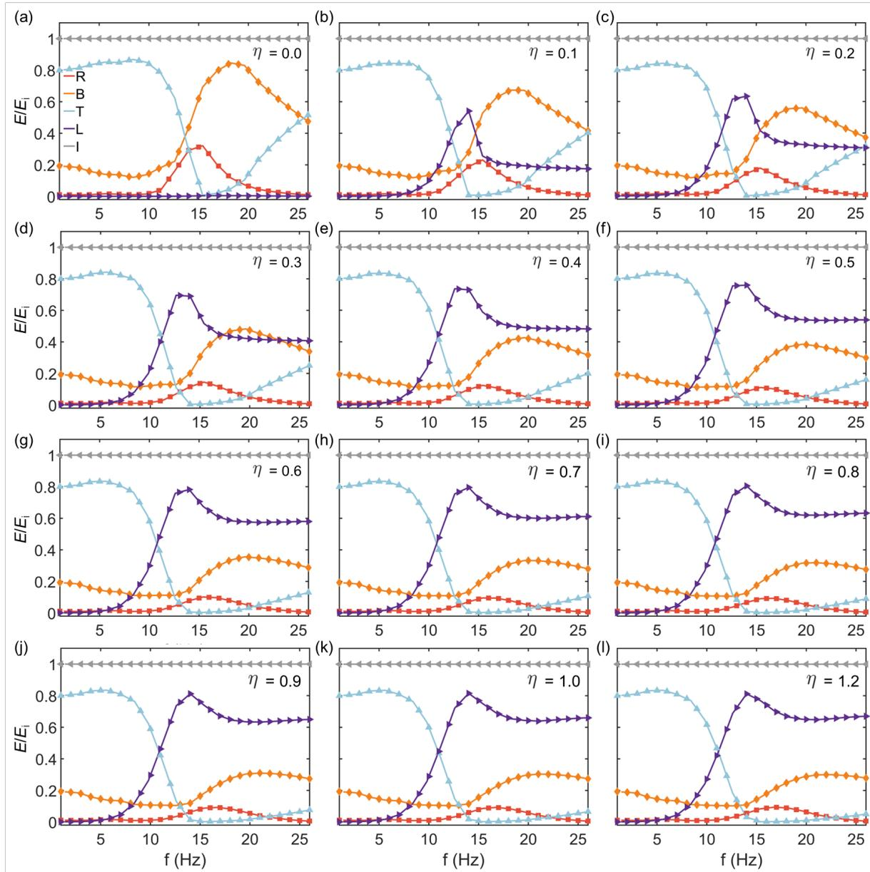
Figure 16: The energy ( $E$ ) normalized by the incident energy is categorized as reflected Rayleigh wave (R), transferred bulk wave (B), transmitted Rayleigh wave (T), resonator absorption (L), and incident wave (I) with respect to different loss factors and different frequencies.  $S_1$ ,  $S_2$ ,  $S_3$ , and  $S_4$  are the regions for calculating the energy of reflected Rayleigh wave, transmitted Rayleigh wave, bulk waves, and absorption by the EDM.
