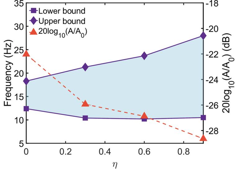
Figure 3: The bandwidth at -10 dB (purple region) and minimum FRF (orange dashed line) in the function of loss factor  $\eta$ . The data are obtained from the right panels of Figs. 2(a-d).
